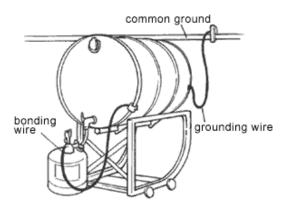
**Assessment of Bonding and Grounding:** Test the resistance of the bonding-grounding connections with an ohmmeter. To prevent the accumulation of static electricity, the total resistance of the grounding circuit should be less than 10 ohms ( $\Omega$ ).
