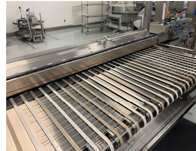
Tubing one table with new process, tubing enters table from cutting equipment to the right
